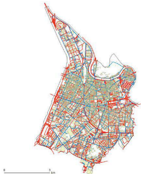
Fig. 68: Grenoble's power network (blue line), road network (red line) and built-up footprints (dotted pastel), see Paper 1752
