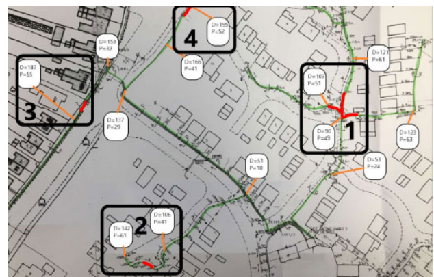
Fig. 5 of paper 837: Impedance contoured plan (D=distance in m, P= phase impedance in milliOhms). Locations highlighted
