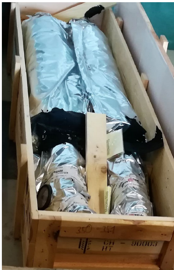
Figure 32 Storage of bushings in a wooden transport box, each sealed with a foil prohibiting moisture ingress
