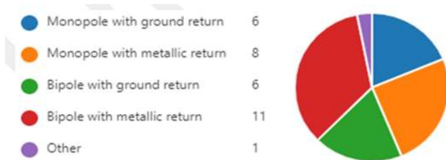
Figure 4.2-9: Different type of Voltage polarity in the DC solutions of the respondents.
