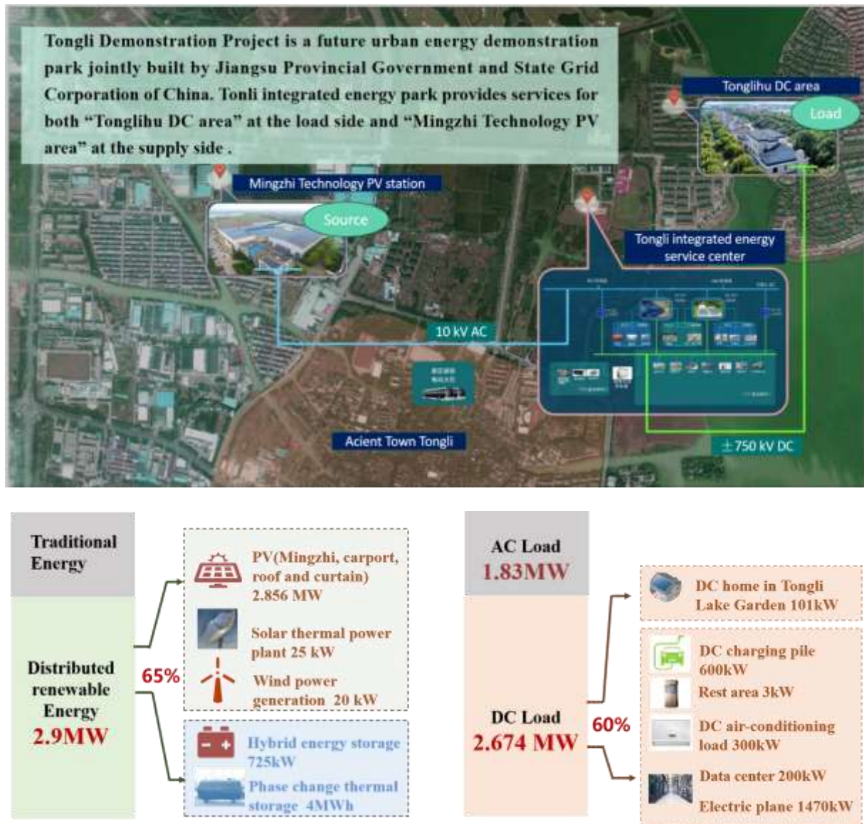
Figure 3.3-10: Suzhou Tongli AC/DC system layout.
