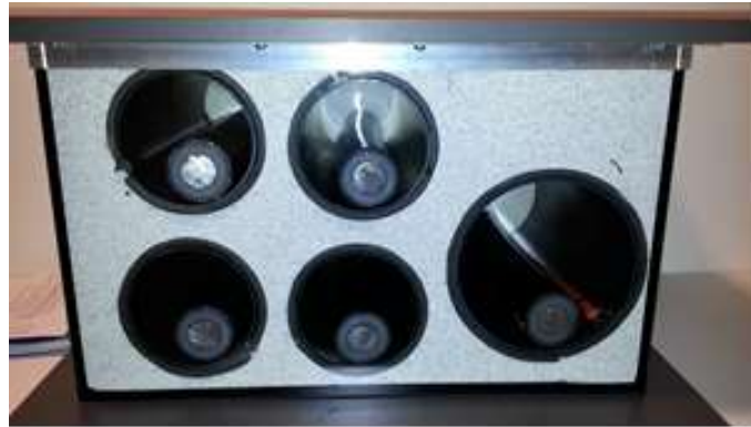
Figure 3.4-23: Cross-sectional model of the underground line, two power strings (left upper and lower pair), neutral and data cables (right).
