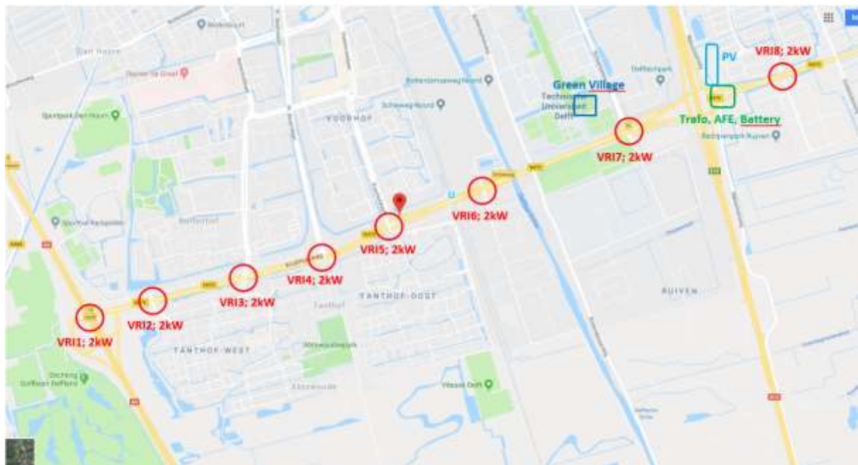
Figure 3.3-29: The layout of the N470 project.
