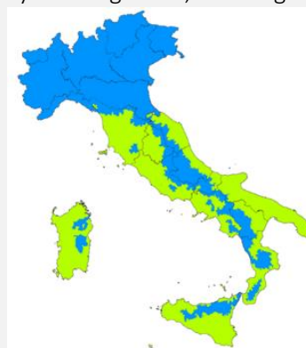
Figure 8 - Italy map with two ice zones, according to Italian Standard CEI 11-4:1998
