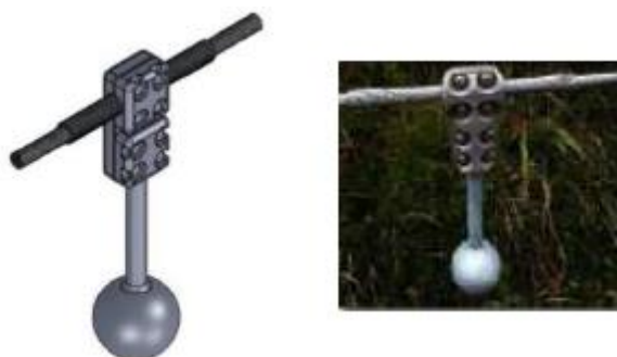
Figure 21 - Anti-rotational device structure and installation layout
