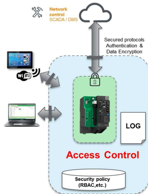
Figure 3: Role Based Access Control & secured protocols
