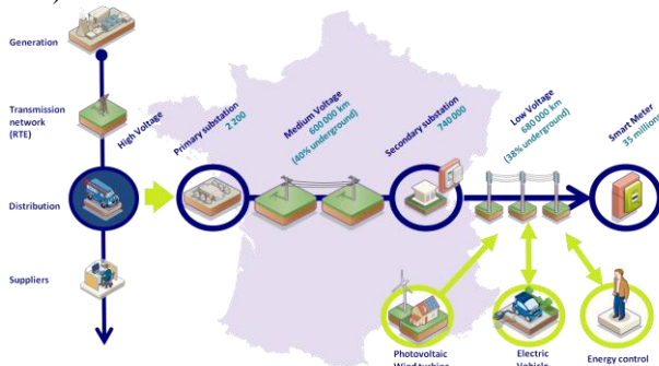
Figure 1 : schematic drawing of networks operated by Enedis
