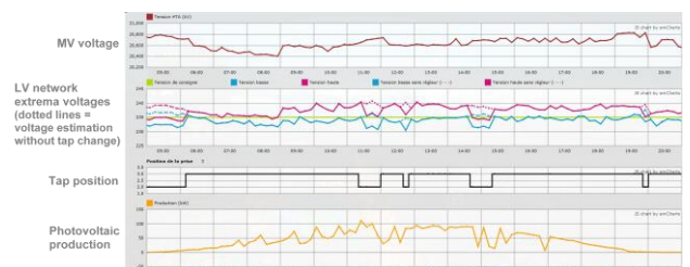
Figure 10 : data collected showing the behavior of voltage regulation on a spring day with variable production.
