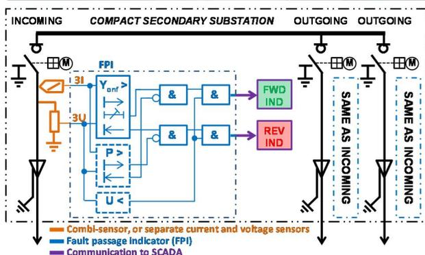
*Fig. 2* Field-tested CSS and its simplified single-line diagram with the novel earth-fault indication functionality.
