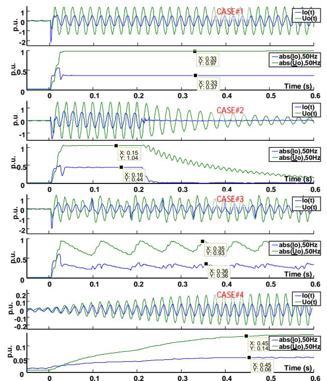
Fig. 5 Example recordings from the field test ( $I_n=80A$ ,  $U_n=11.547kV$ )
