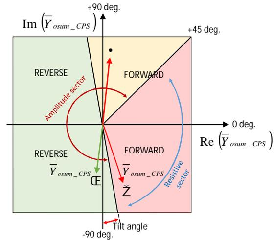
*Fig. 1* Illustration of the directional characteristics of the MFA-function.
