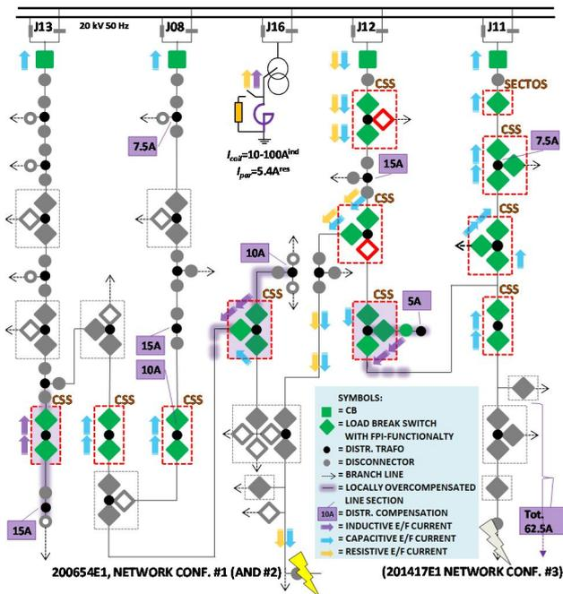
Fig. 3 Simplified single-line diagram of the Orivesi test network with principal fault current flow in the CSSs (faulty feeder J12).
