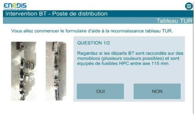
Figure 5: Assisted recognition of LV panel type
