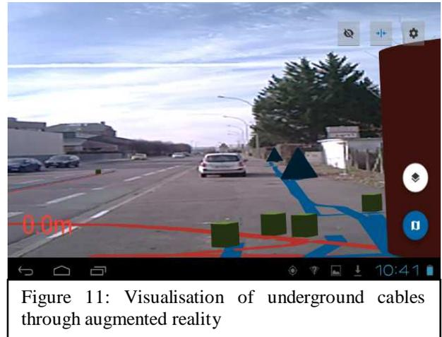
Figure 11: Visualisation of underground cables through augmented reality
