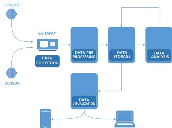
Figure 2 Information flow in the ABB Ability™
