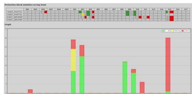
Figure 5 Statistics on analyzed fault cases
