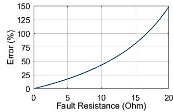
Fig. 14. di/dt error with fault resistance in the location 1 P-P fault condition.
