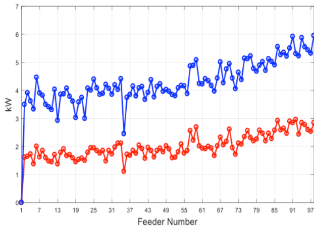
Figure 6: A comparison of the feeder index (50% EV uptake). Blue: Mini-E trial, red: My Electric Avenue trial. Note that an adjustment is made to the My Electric Avenue dataset to reflect 7.4kW chargers being used, which is consistent with the Mini-E trial. This adjustment applies the same start-of-charge times as the 3.7kW chargers from the My Electric Avenue trial and the ‘on-time’ is reduced by approximately half (rounded up to the nearest half hour)
