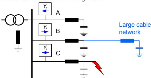
Fig. 5 Direction of 5<sup>th</sup> harmonic, if the series resonance frequency is higher than the 5<sup>th</sup> harmonics
