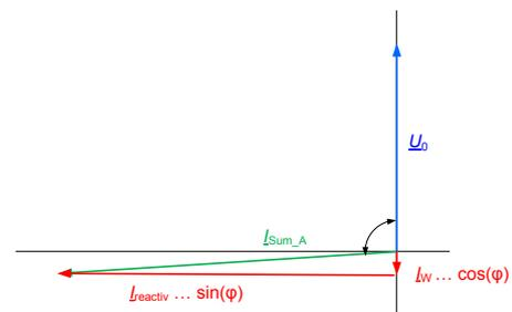
Fig. 3 Directional identification of the faulty feeder at 50 Hz
