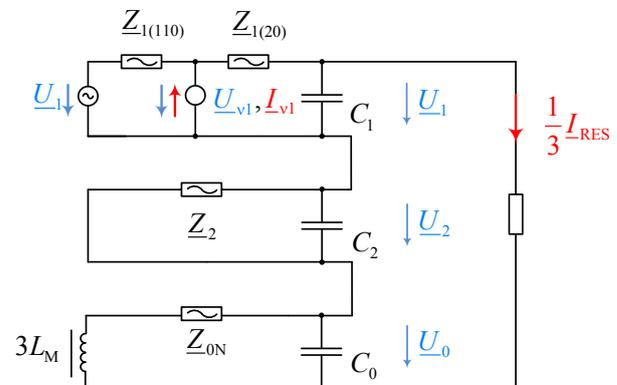
Fig. 7 Simplified equivalent circuit in symmetrical-components considering the 110-kV-network in case of a single-phase earth fault [6]
