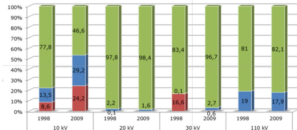
Fig. 1 Neutral Point Treatment in Germany [4]: green: Petersen-Coil; blue: solid grounded; red: isolated
