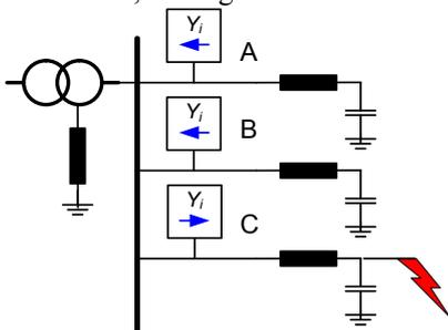
Fig. 4 Directions of 5<sup>th</sup> harmonic, if the series resonance frequency is below the 5<sup>th</sup> harmonics
