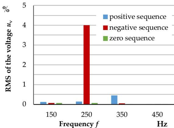
Fig. 8 Measured phase to earth voltage at the bus bar before earth fault [6]
