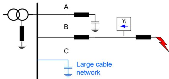
Fig. 6 Direction of 5<sup>th</sup> harmonic in distributed relays, if the series resonance frequency of feeder and base network is higher than the 5<sup>th</sup> harmonics
