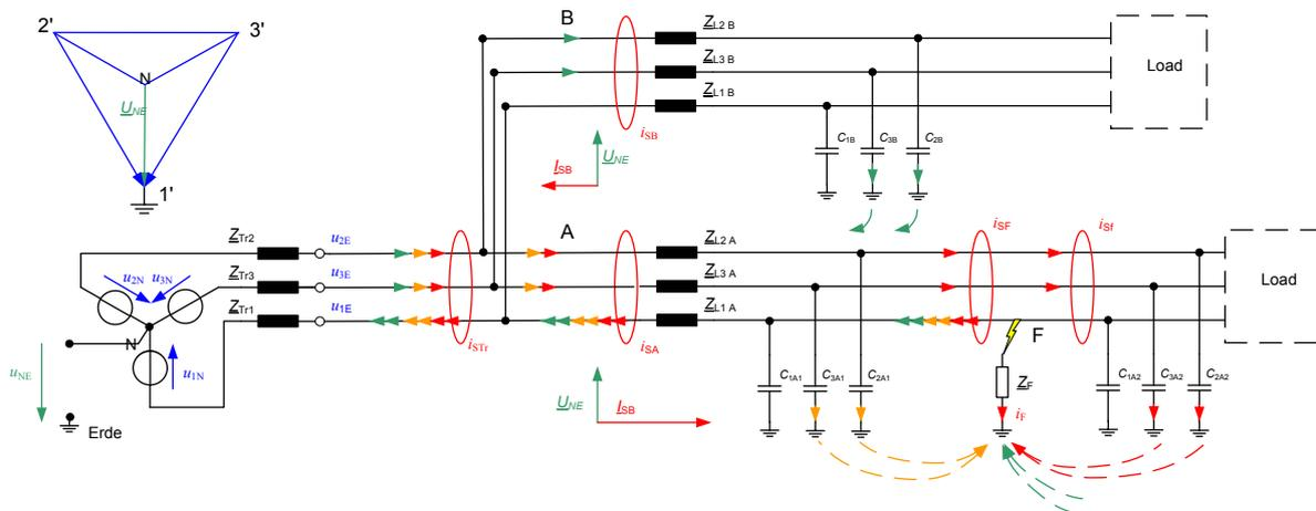
Fig. 2 Single-line-earthfault (SLE) in feeder A of the isolated network
