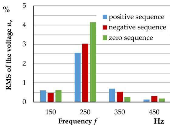
Fig. 9 Measured phase to earth voltage at the bus bar during earth fault [6]
