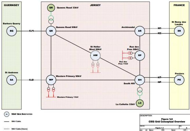
Figure 3. Conceptual representation of the Electrical Grid
