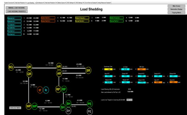
Figure 4. Operator HMI. Example of Split mode.
