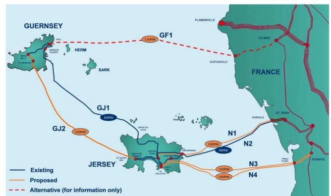
Figure 1. Electrical Grid. Existing and Future Grid
