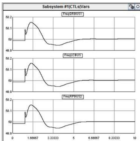
Figure 6. Frequency after load shed
