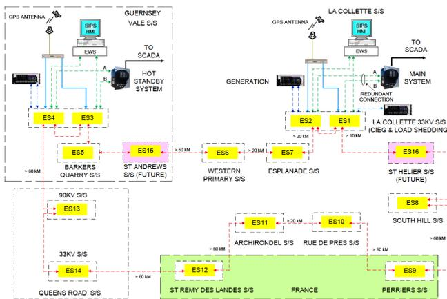
Figure 5. Hardware Architecture implemented
