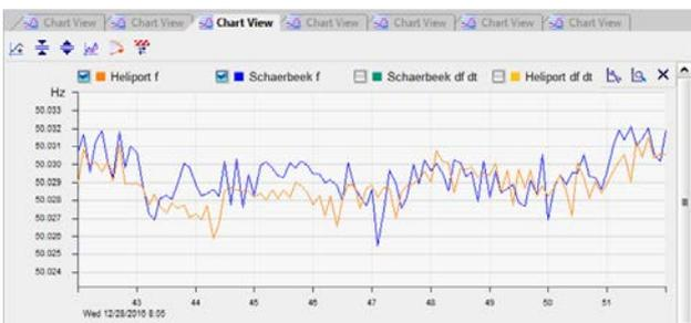
**Figure 8:** Example for frequency measurements from PMUs
