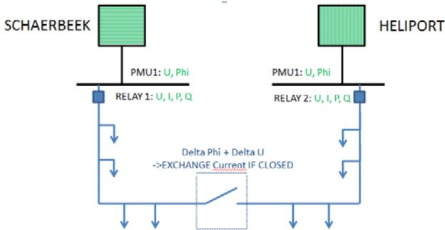
**Figure 5:** Scheme for supervision of phase angle
