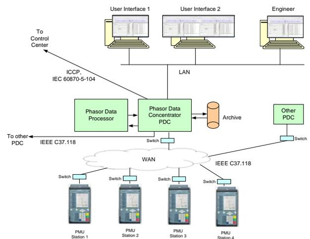
**Figure 1:** Structure of a Wide Area Monitoring System
