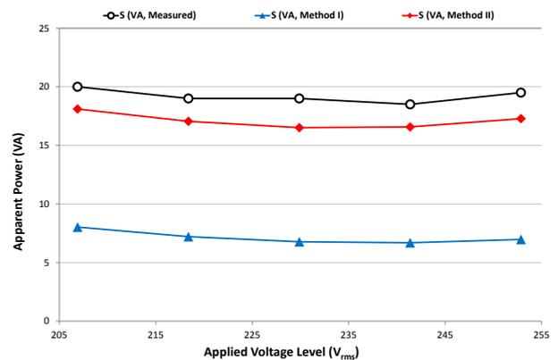
**Figure 4: Measured and Estimated Apparent Power vs Applied Voltage (Test C,  $THD_V = 5.0\%$ )**
