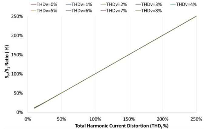
**Figure 1: Apparent Power Ratio ( $S_N/S_1$ ) vs Current Distortion, for different levels of Voltage Distortion**
