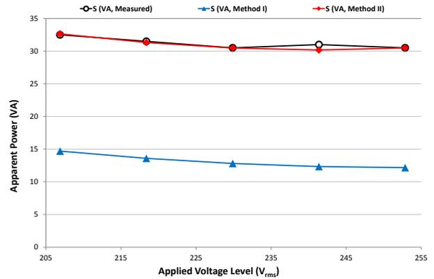
**Figure 2: Measured and Estimated Apparent Power vs Applied Voltage (Test A,  $THD_V = 0.0\%$ )**
