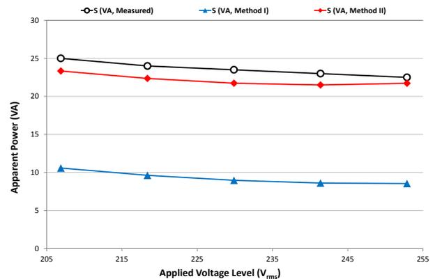
**Figure 3: Measured and Estimated Apparent Power vs Applied Voltage (Test B,  $THD_V = 2.5\%$ )**
