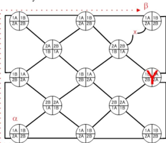
**Figure 4.** After equipment failure (Y), another route is automatically taken.
