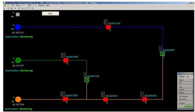
**Figure 6.** Normal condition. Red squares are normally closed reclosers, green squares are normally open reclosers (ties) and circles are substation circuit breakers.
