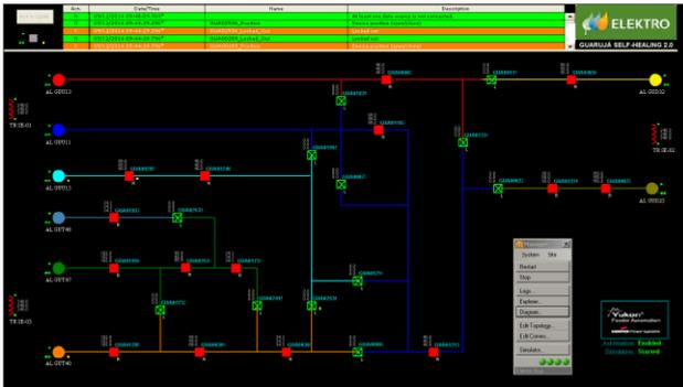
**Figure 13.** Screenshot from the automation server with part of the reclosers – segmented MV network with many possible automatic operations and load analysis in real-time
