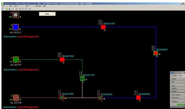
**Figure 10.** After a while, load increases again and there is no option unless shedding part of the load, avoiding again a substation or conductor overload.
