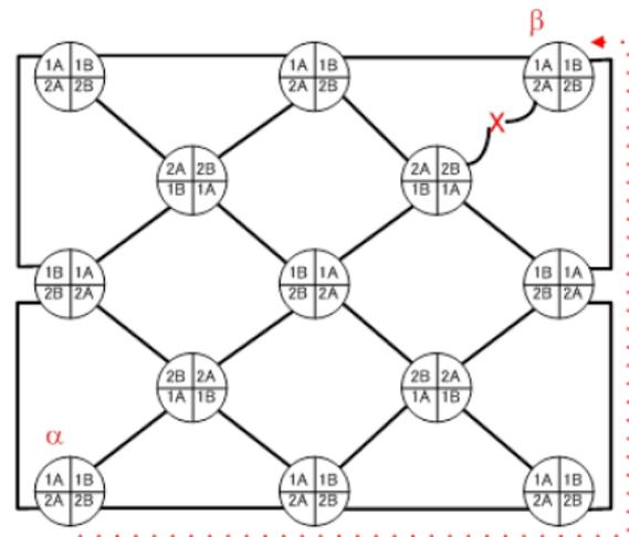
**Figure 3.** After the cable was brake (X), another route is automatically taken.
