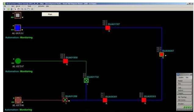
**Figure 8.** Fault is located, isolated and the service is restored by a tie point.
