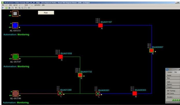
**Figure 9.** After a while, load increases and another tie is closed to split the load, avoiding an overload at the substation or at a conductor.
