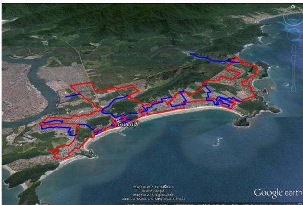
**Figure 1.** 85 km fiber optics pathway after project deployment on February 2016 – all the data is directed to the regional office where is located the automation server and the data link to the Operational Center in Campinas,
