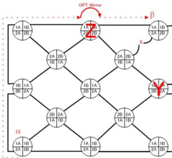
**Figure 5.** After an equipment power outage (Z), the optical bypass is activated keeping the route alive.
