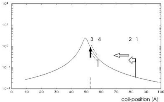
Fig. 1: Standard control method by coil adjustments in order to calculate resonance curve and network parameters.
