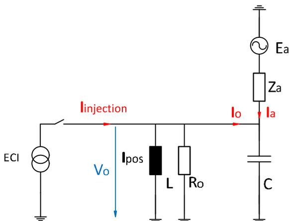
Fig. 2: Control method with 50 Hz current injection for calculation of network parameters.
