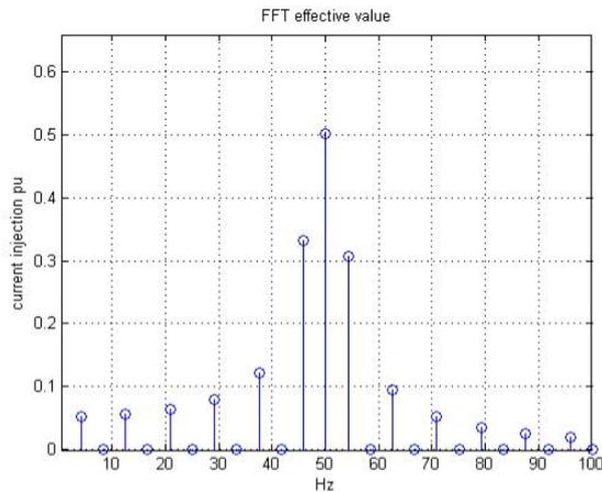
Fig. 4: Frequency spectrum caused by pulsed injection pattern.
