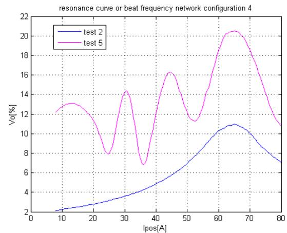
Fig. 8: Network configuration 4, test 2 and test 5 measured voltage over coil position
