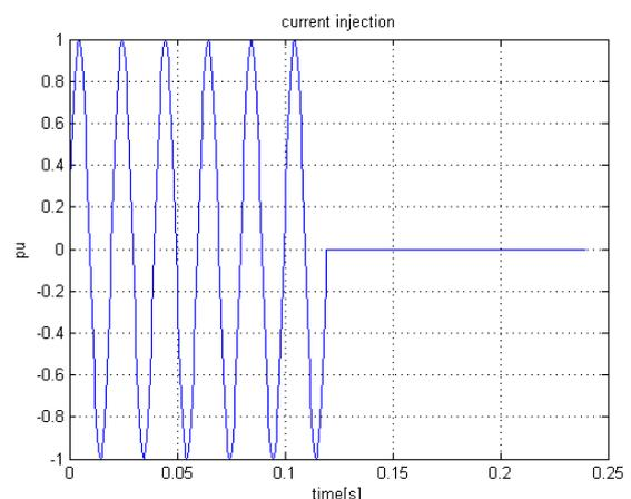
Fig. 3: Current injection pattern for generation of side bands to the 50 Hz main frequency.
