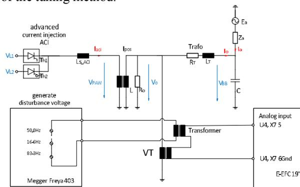
Fig. 6: Test arrangement for interference test
