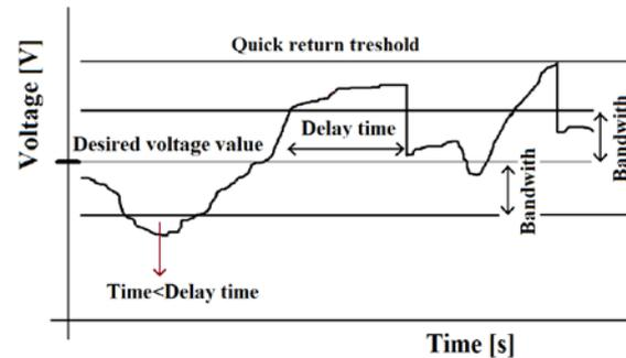
Fig. 10 The principal of the voltage regulation algorithm
