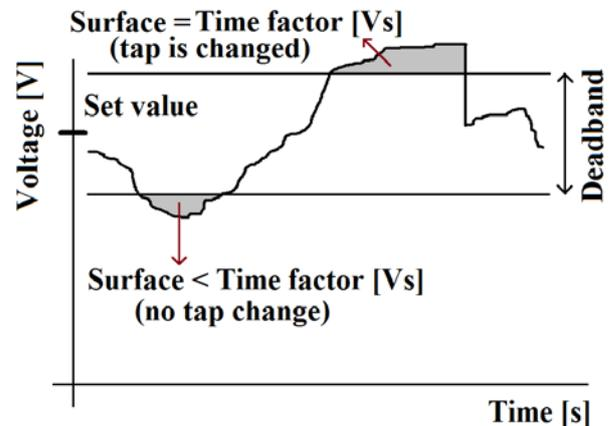
Fig. 8 The principal of Stage 1 control algorithm
