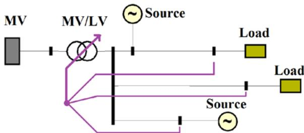
Fig. 4 The principal of voltage regulation
