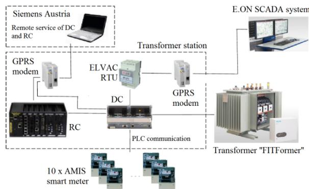
Fig. 6 Logical architecture of the regulation
