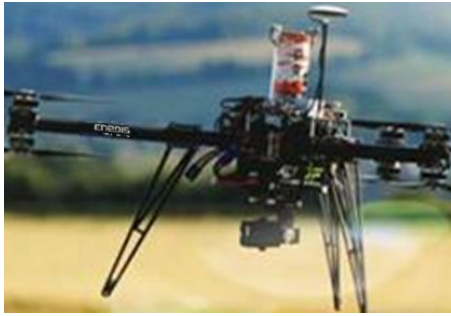
Figure 5 Drone operated by Enedis for MV overhead power lines maintenance
