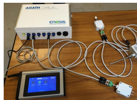
Figure 4 Enedis HV/MV transformers monitoring solution
