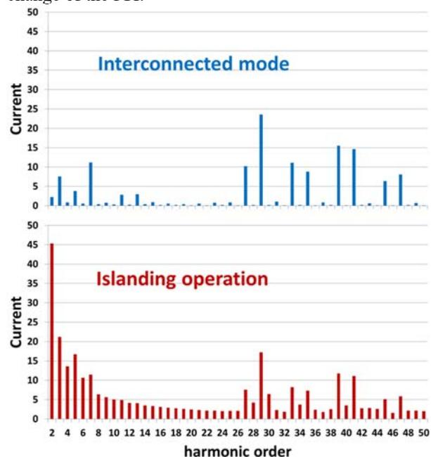
Fig. 9: Harmonics of the converter current in interconnected and islanding operation
