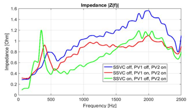
Fig. 4: Change of the frequency dependent grid impedance related to the amount of connected PV systems and the upstream (SSVC).
