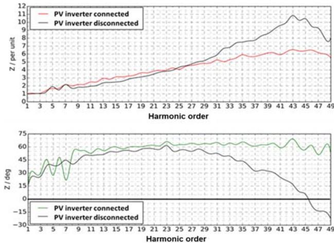
Fig. 2: Influence of 30 parallel, similar inverters ( $S_{equ} = 930$  kVA) connected to a strong grid point ( $Z@50\text{Hz}$  PV-inverter off =  $0.059$  ohm,  $Z@50\text{Hz}$  PV-inverter on =  $0.064$  ohm) (Upper diagram: Amplitude in per unit, Lower diagram: phase or argument absolute)
