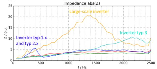
Fig. 3: Grid impedance measurements in inverter dominated grids at different PCC.
