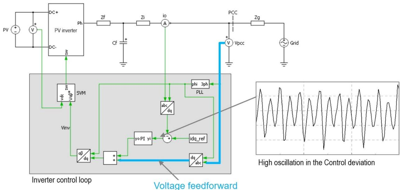
Fig. 6: PV inverter control loop with the voltage feedforward
