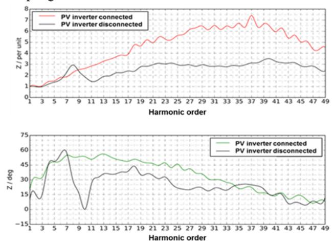
Fig. 1: Influence of three parallel inverters ( $S_{\text{equ}} = 56 \text{ kVA}$ ) connected to a weak grid ( $Z@50\text{Hz PV-inverter off} = 0.259 \text{ ohm}$ ,  $Z@50\text{Hz PV-inverter on} = 0.314 \text{ ohm}$ ) (Upper diagram: Amplitude in per unit, Lower diagram: phase or argument, absolute)
