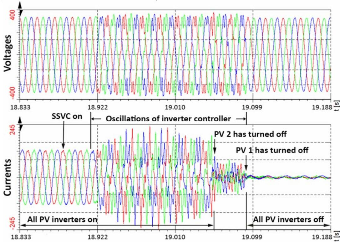
Fig. 5: Voltage and current on the output of the SSVC when the SSVC is connected
