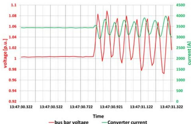
Fig. 8: RMS values of grid voltage and converter current while switching in islanding operation
