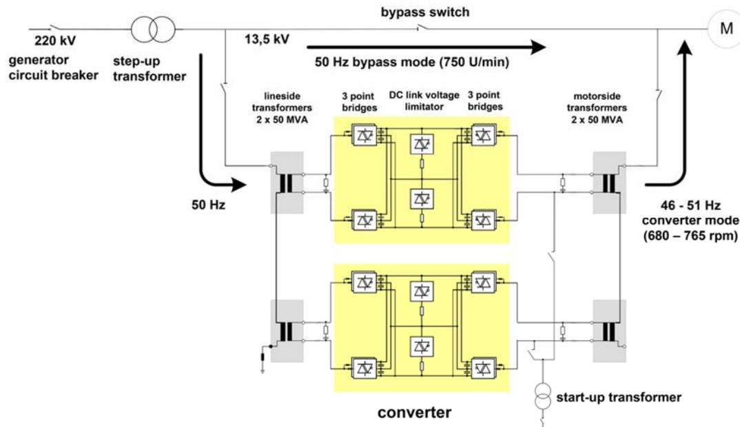
Fig. 7: Single line diagram of the converter Grimsel 2 [4]
