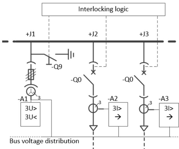
Figure 3. Reference application with bus voltage sharing and interlocking using hard-wired signals.
