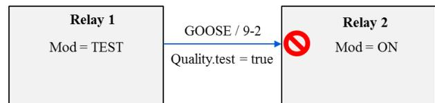
Figure 1. IEC 61850 mode handling in protection relay
