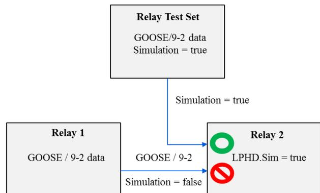
Figure 2. Simulation according IEC 61850
