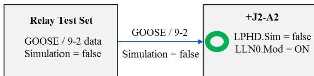
Figure 4. Periodical relay testing by connecting test set directly to the relay.
