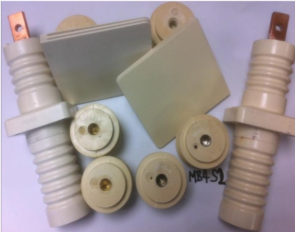
Figure 4. Example demonstrator components cast from masterbatch nano-micro composite material formulations.
