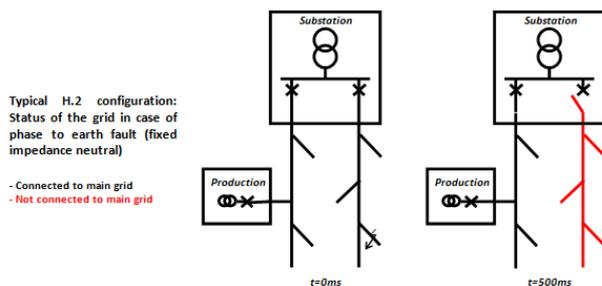
If a severe phase to phase short circuit happens (for example three phase fault not far from producer location), the voltage dips causes the tripping of the H.2 relay (same as H.1).
