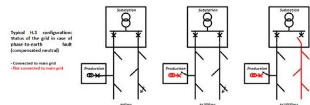
Grid access quality is low for production with H.1 settings. It can be sufficient for small production where a high number of tripping is not a problem. The situation may however be improved using delays in the settings.
