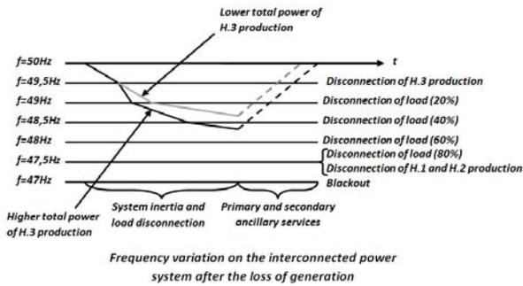
As a consequence, Enedis changes the narrow settings (47.5Hz/51.5Hz) when the rate of change of frequency (ROCOF) is below 0,5 Hz/s (the frequency drop/rise is slow, which means the generator is likely to be connected to the main power system). When the frequency drop/rise is higher than 0,5 Hz/s, the generator is supposed to be connected to a feeder which is disconnected from the transmission grid, and disconnection occurs when frequency is outside the narrow settings (49.5Hz/50.5Hz).
