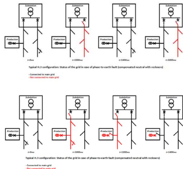
Note that this behavior is not certain if the situation on the islanded feeder is close to equilibrium when the fault appears. This combination of H.3 protection and fast reclosers works in most cases, and thus allows a minimum impact of faults on the quality of supply.
