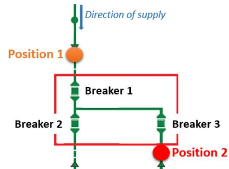
Figure 2 – A diagram of the two possible FCI installations in terms of position relative to the breakers.
