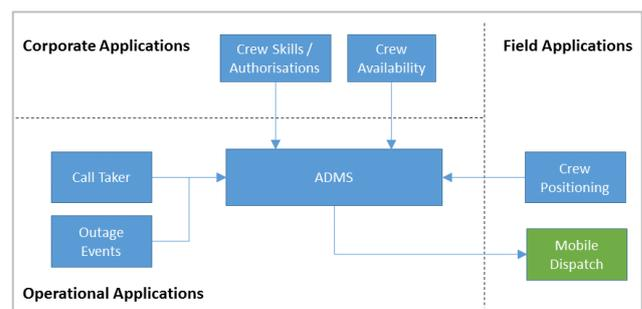
Figure 1 - High-level blocks of auto-dispatch mechanism
