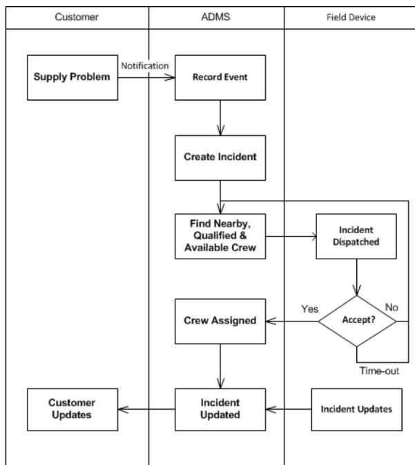
Figure 2 - Workflow for Auto-Dispatch of Fault Work
