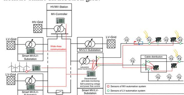
Fig. 1: Possible structure of a holistic automation system for low and medium voltage grids
