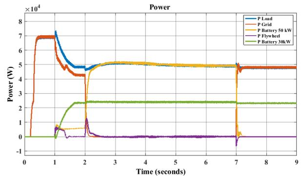
Figure 3 – Active power profile on the grid on transition grid-connected/islanding operations
