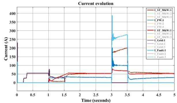
Figure 7 - Phase to ground fault on the LV busbar, islanding mode
