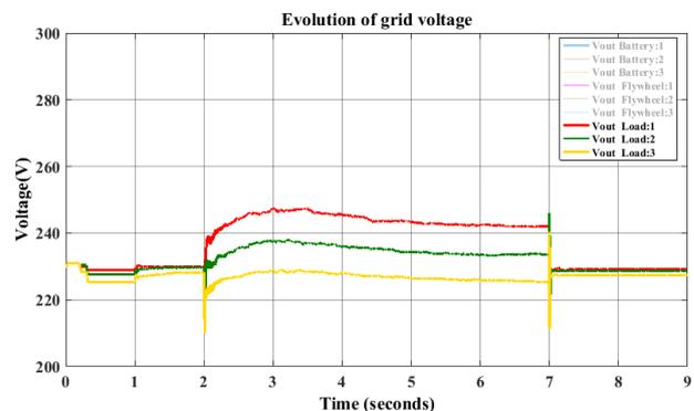
Figure 5 – Voltage profile on the grid on grid-connected/islanding operations
