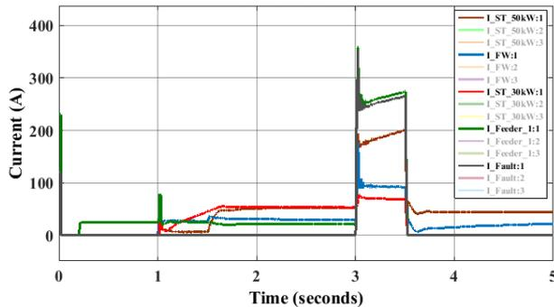
Figure 9 - Phase to ground fault on feeder 1, 200 m from the secondary substation, islanding mode
