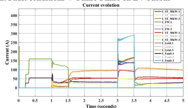
Figure 8 - Phase to phase fault on the LV busbar, islanding mode
