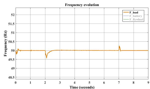
Figure 4 - Frequency profile on the grid on transition grid-connected/islanding operations
