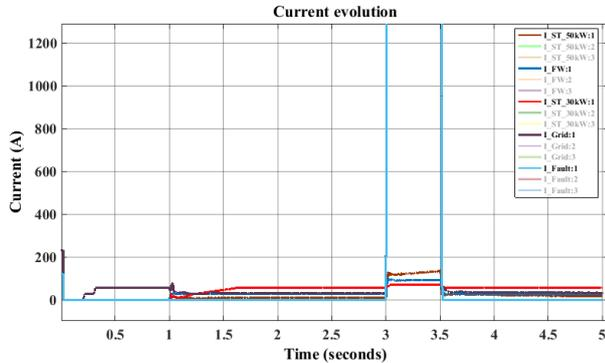
Figure 6 – Phase to ground fault on the LV busbar, grid-connected mode
