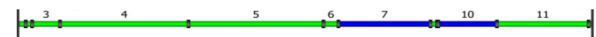
Figure 3: Schematic display of the 1335m long cable, green XLPE cable, blue is PILC cable
