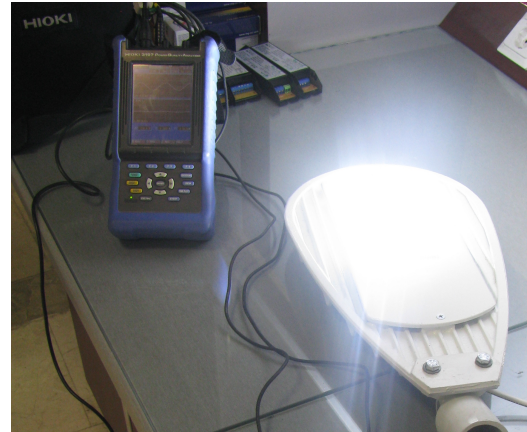
Fig. 2: experimental test using a power quality analyzer.
