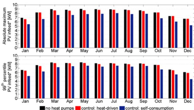
Figure 4: Absolute maxima and 99<sup>th</sup> percentiles of the sum of the PV power and the power demand of the heat pump (\*: PV infeed without remaining load of household)
