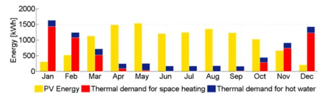
Figure 1: Electric energy production by a PV unit and thermal energy demand for space heating and hot water for an exemplary household
