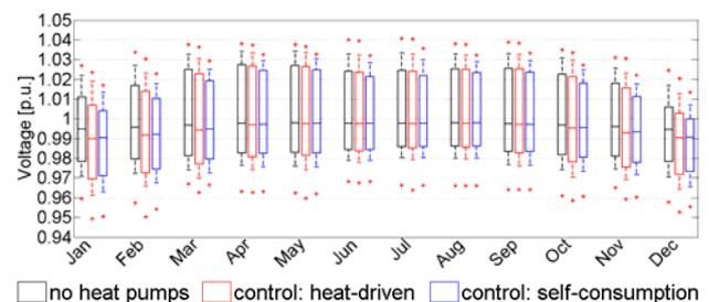
Figure 5: Results of load flow simulation for a penetration rate of heat pumps equal to 20%
