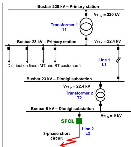
Fig. 3. Grid layout for the 3-phase fault event
