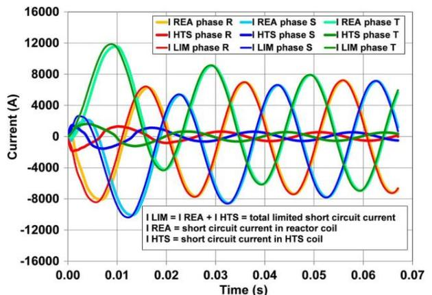
**Fig. 5.** Limited short-circuit current ( $I_{LIM}$ ): comparison between the current flowing through the HTS windings ( $I_{HTS}$ ) and the reactors ( $I_{REA}$ ).
