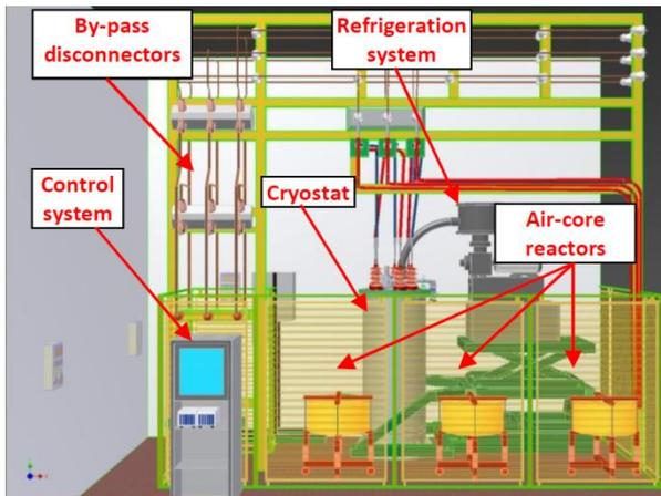
Fig. 1. General sketch of the SFCL grid installation
