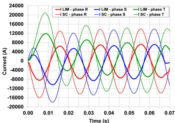
**Fig. 4.** Time behaviour of the prospective fault current without SFCL ( $I_{SC}$ ) and of the fault current as limited by the SFCL device ( $I_{LIM}$ ).
