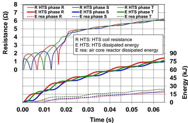
Fig. 6. HTS windings resistance and dissipated energies of air-core reactors and HTS windings during the fault transient.
