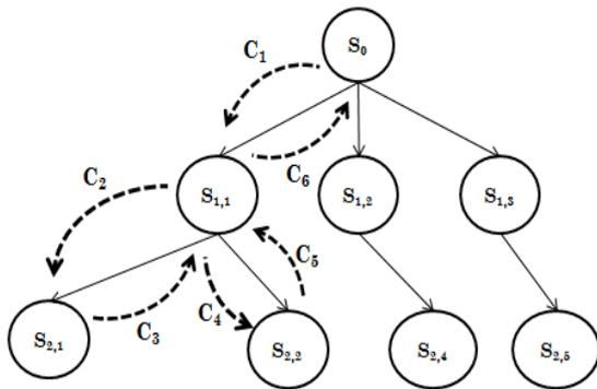
Figure 1: Branch-and-bound algorithm execution
