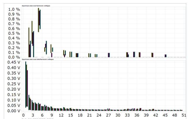
Figure 1: Harmonic- and interharmonic voltages when the wind turbine is disconnected. The highest value is from the 5. harmonic voltage.
