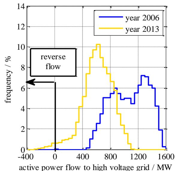
**Figure 1:** Histogram of active power flow between the distribution and transmission grids (negative values represent power export from the distribution grid)
