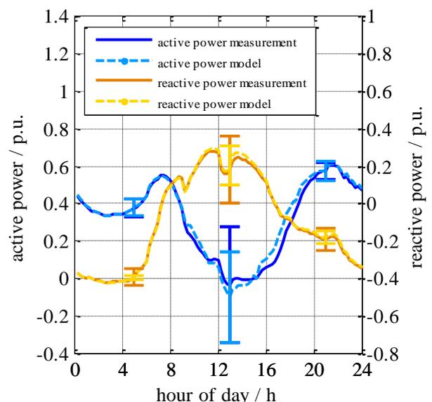
**Figure 3:** Measurement and model of active and reactive power flow at one substation (negative values represent power flow from the MV-grid to the 110kV grid)
