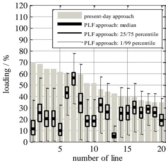
**Figure 4:** Line loadings in the present-day and hybrid (probabilistic) planning approach
