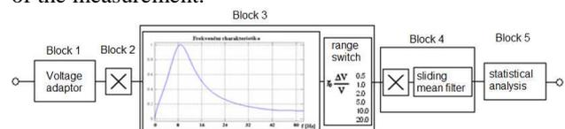
Figure 1: Block diagram of flicker-meter
