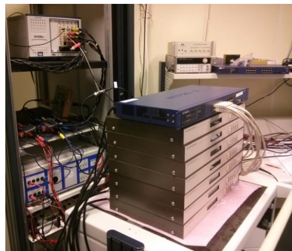
Figure 3. VSL system for PMU testing.
