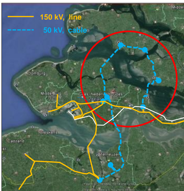
Figure 1. Geographic layout of the DNWG 50 kV grid (blue dashed line), with the northern part marked by a (red) circle. The 50 kV substations are marked with dots.
