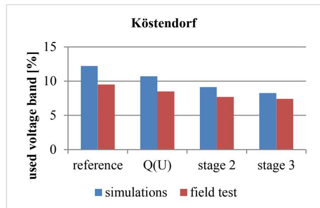
Figure 3 Voltage band usage in Köstendorf
