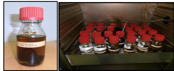
Figure 2: ageing at 130°C in 25ml glass vessels with air blanket and inhibited mineral oil
