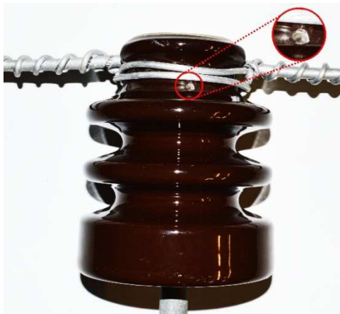
Fig. 4: Insulator with a hole drilled from the side to the locking pin, simulating an electrical puncture.
