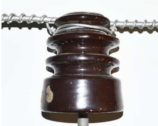
Fig. 3: Insulator sample taken from the grid, with actual contamination preserved.
