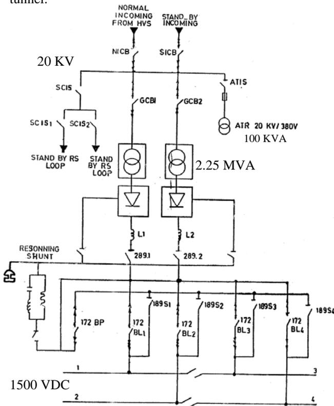
Fig. 1 Rectifier station diagram
