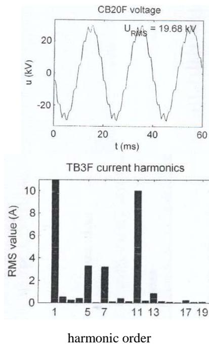
Fig. 3 Measured  $V_{pcc}$  waveform and harmonic for RS
