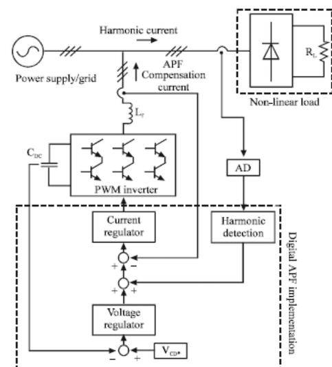
Fig. 5 System modeling of active harmonic filter by micro controller model
