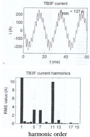
Fig. 2 Measured  $I_s$  waveform and harmonic spectrum for traction bus-bar # 3F "TB3F"
