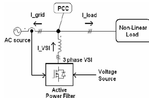
Fig. 4 Shunt active filter single line diagram
