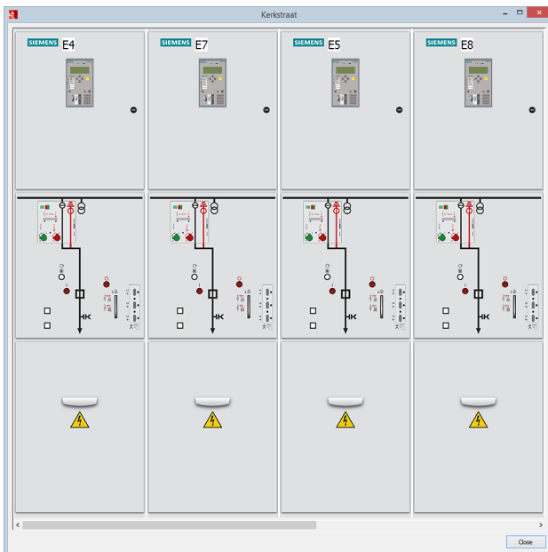
Figure 9. Switchgear installation with position indication and protection relay indications
