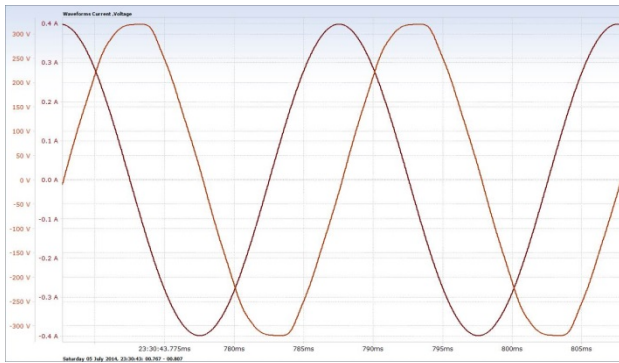
Figure 3 Voltage and current measured at the terminal of an inverter during no production
