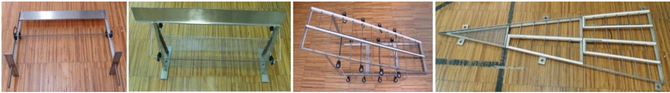
Fig. 11 - Electrified structures in test. From left to right: vertical; prism; oblique and oblique for metal pole
