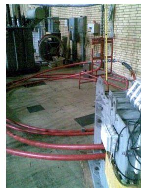
Figure 2 Type testing of 10kV cable
