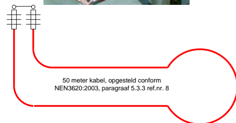
Figure 2 Type testing of 10kV cable
