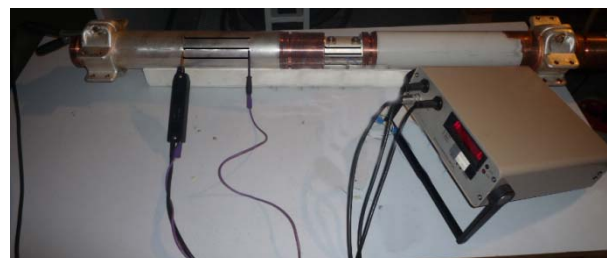
Fig. 6: Test setup for the evaluation of the current homogeneity
