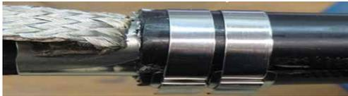
Some observed failures are due to incorrect installation of the metallic connection devices. As the cable and accessories are often delivered separately by different manufacturers, the compatibility of different designs is also in question.
